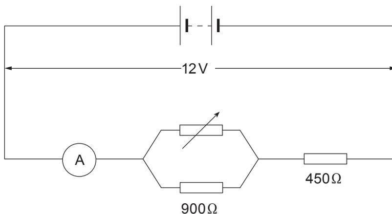
The variable resistor is adjusted so that the ammeter reads 0.01 A.
